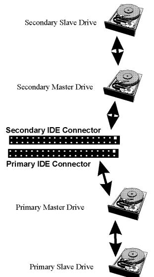
**Attach IDE Cable J11** is the primary IDE (Integrated Drive Electronics) hard disk drive connector. Both the primary master and the primary slave IDE drives must be connected by cable to J11, as shown below.
